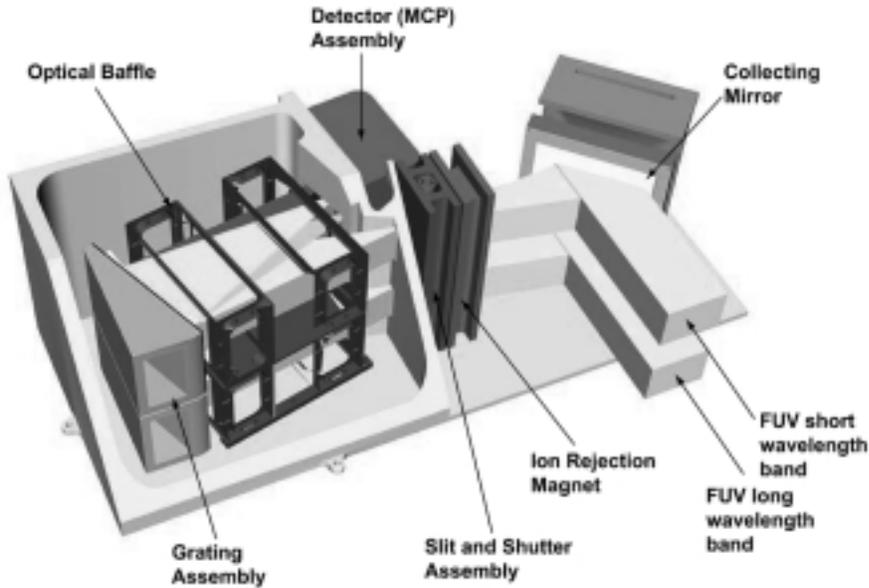
**Figure 2.** Three dimensional schematic diagram which represents the mechanical design of the FIMS system
