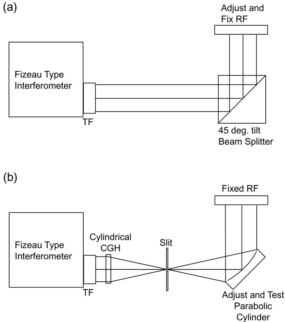
**Figure 6.** Procedure of testing an off-axis parabolic cylinder mirror using a beam-splitter to reduce the degree of freedom which utilize the angle of the reflected beam from a beam-splitter is  $90^\circ$ . (a) shows the preliminary procedure to fix the reference flat mirror in a proper position using the beam-splitter. (b) is the optical setup where the off-axis parabolic cylinder mirror is adjusted to make a fringe pattern. The setup is not tolerant to the error in the off-axis angle.
