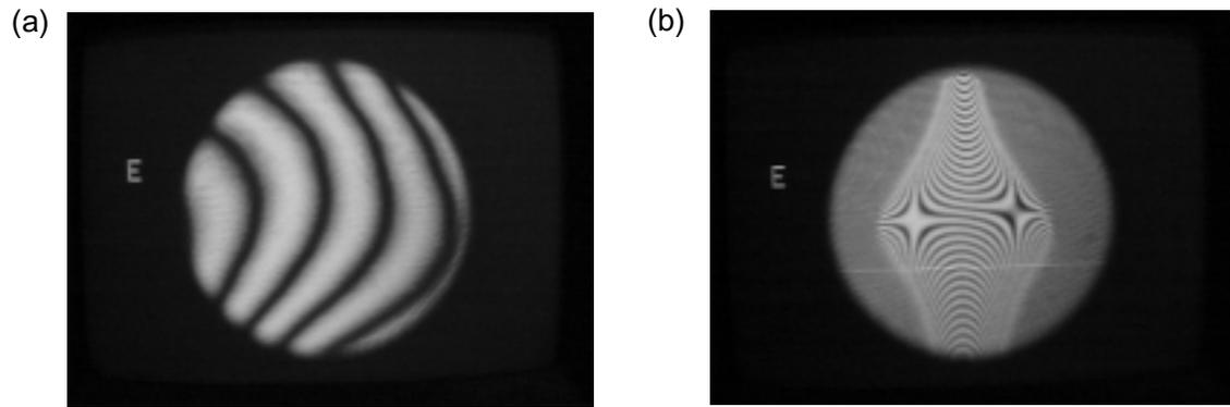
**Figure 4.** Interference pattern when a flat mirror is located at the focal line of the CGH. The converging beam(a) and the diverging beam(b) generate different interference patterns
