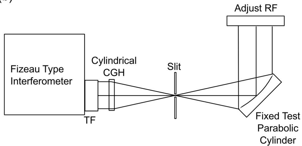
**Figure 7.** Procedure of testing an off-axis parabolic cylinder mirror using a retro-reflector to reduce the degree of freedom which has a tolerance in off-axis angle of the mirror. (a) shows the preliminary procedure to fix the off-axis parabolic cylinder mirror in a proper position using the retro-reflector. (b) is the optical setup where the reference mirror is adjusted to make a fringe pattern.
