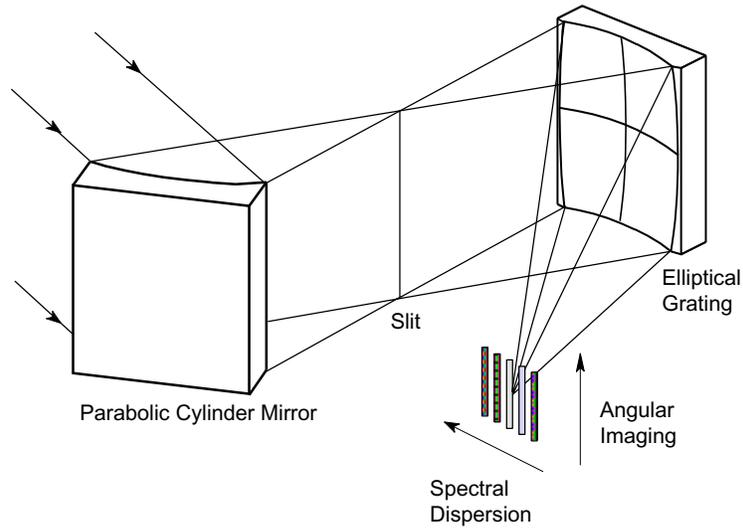
**Figure 1.** Schematic diagram which represents operation principle of FIMS
