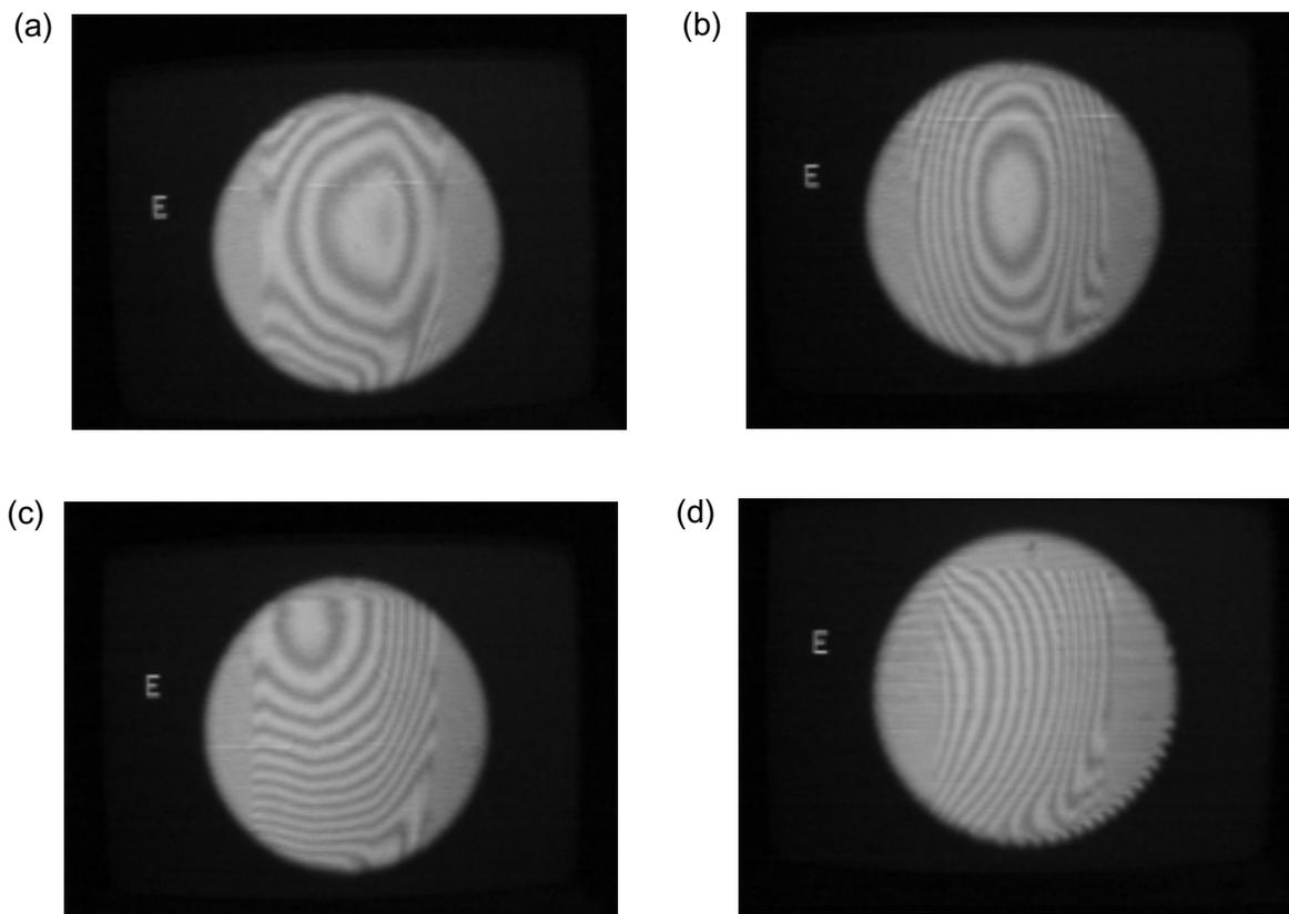
**Figure 5.** Interference patterns of the standard on-axis cylindrical mirror. (a) is the interference pattern when the mirror is adjusted to minimize fringes. (b) is the change of the pattern as the mirror is translated along the z-axis(optical axis). The pattern of (c) and (d) are the changes of the pattern when the mirror is tilted about the x and y axis respectively.
