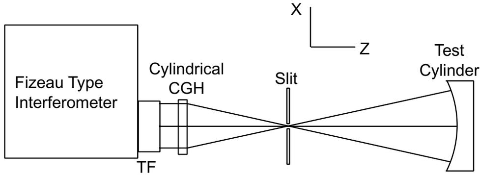
**Figure 3.** The optical setup for measuring the standard on-axis parabolic mirror using the cylindrical CGH
