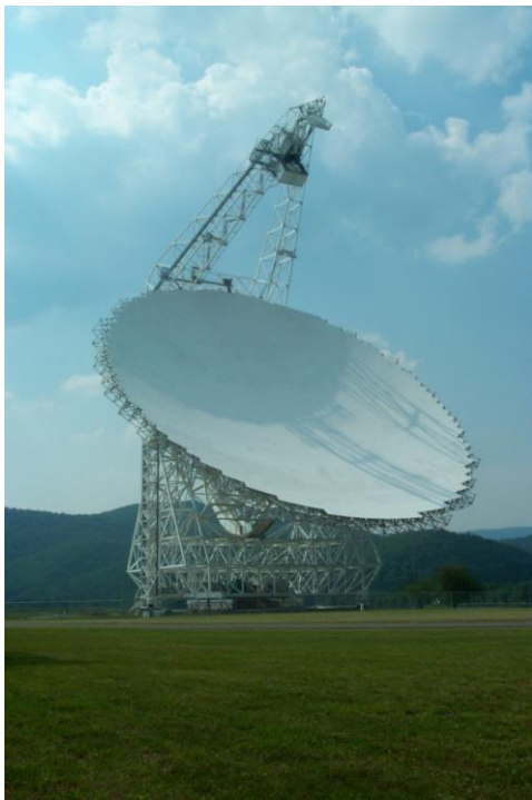
Figure 9: The National Radio Astronomy Observatory’s Robert C. Byrd telescope in Green Bank, West Virginia, utilized by the University of California Berkeley’s eavesdropping and panchromatic SETI projects. The 100 meter diameter telescope is the largest fully steerable radio telescope on the planet, and with observing capabilities extending up to 100 GHz.
